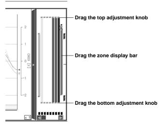
You can change the waveform display zone on the trend display screen by clicking the edit zone icon or by selecting [Y-Axis] - [Edit Zone].
