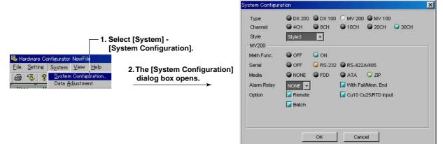
Only the system configuration in the setup data file can be checked. If the system configuration is changed and the [OK] button is clicked, a message "System Configuration is changed Input & Data are Initialized" appears. Clicking the [OK] button initializes the data.
