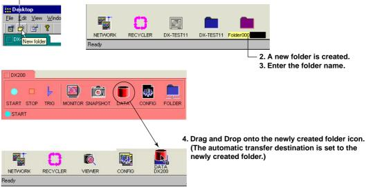
The data residing in the internal memory or external storage medium of the DX/MV can be automatically transferred to the specified folder on the PC.
