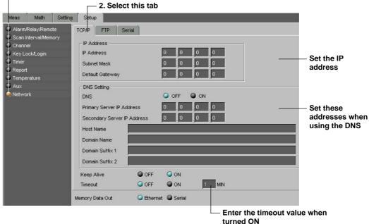
In the case of a CONFIG file, the IP address cannot be configured. When communicating with the DX100/DX200/MV100/MV200 via Ethernet, the IP address, subnet mask, and default gateway must be set on the DX100/DX200/MV100/MV200 beforehand.
