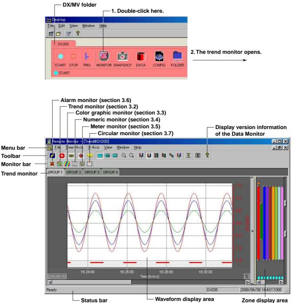
The Data Monitor can be used to monitor the measured/computed data and the alarms of the DX100/DX200/MV100/MV200. The following six monitoring methods are available:
