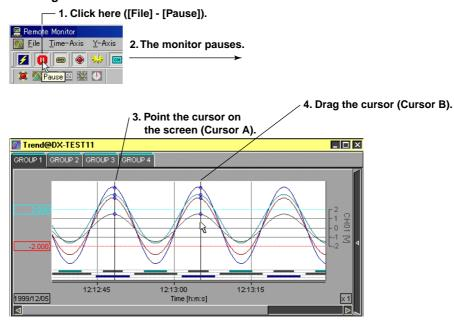
When the mouse is pointed on the screen, Cursor A and Cursor B are overlapped. Cursors can be displayed only when the monitor is paused. Pause the monitor before pointing the cursor on the trend screen.
