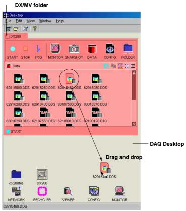
You can copy the file that is located in the DX/MV to the DAQ Desktop by dragging and dropping the file onto the DAQ Desktop.
