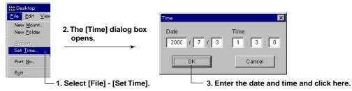
Sets the date and time of all mounted DX100s, DX200s, MV100s, and MV200s at once.
