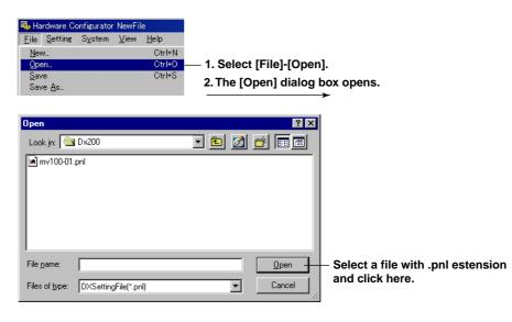
You can specify the location where the setup data file is located and open the Configurator.
