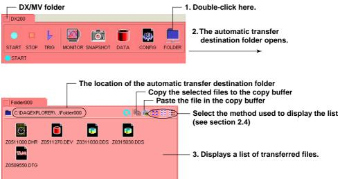
You can also open the above folder by double-clicking the automatic transfer destination folder located on the DAQ Desktop.
