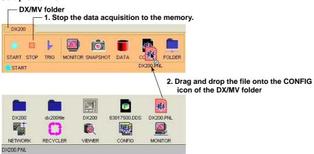
The contents of the setup data file (\*.PNL) located on the DAQ Desktop can be transmitted. If the DX100/DX200/MV100/MV200 is acquiring data to the memory, the data will not be sent in this case.
